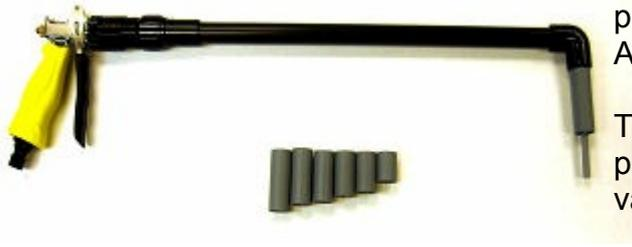
The total length of the filling pistol is 625 mm and it is supplied with a kit of eight spacer tubes so that the probe depth can be accurately set to suit the ranges of Alcad And Saft cells.
